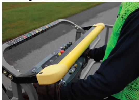
Figure 2: A pressure sensing device positioned over the control panel.
