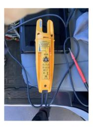
**Event:** Work activity conducted without hot work controls ie. Hot work checklist, gas testing, etc. Contractor performing work activity requiring the use of a battery operated multi meter inside the hazardous area. Not rated for use in a hazardous are (certified to IEC 60079-11)
